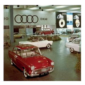
A convertible version of the DKW F 12 was also on display at the Auto Union stand in autumn 1963. The development work had been done by the bodywork company Baur in Stuttgart, which also supplied the full soft top as a complete module.
