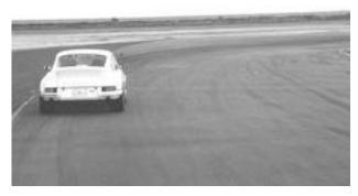
The turn has a depression at the apex, which will unsettle the car, letting it go and then grabbing it again. This results in a slightly jerky feel to the turn, even when it is done optimally. As this turn connects two straights, a slightly late apex is needed to avoid losing substantial time on the ensuing straight. Move the car slightly into the berm,
