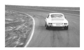
Then apply strong braking, which will take the car past the first apex to the outside portion of the tight part of the turn. 2<sup>nd</sup> gear will be needed before the next car rotation.
